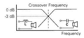
**Coil (L):** Passes low frequencies and blocks high frequencies. (Low pass)
